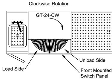
**2. ROTATION:** Conveyor rotation can be clockwise or counterclockwise. The rotation selection is based on work flow. In an underbar environment, the wet waste sink should be on the load side of the glasswasher to prevent crossover (see underbar plan view). In a pass-thru style cocktail station, the load side should be toward the servers (see pass-thru station plan view).
