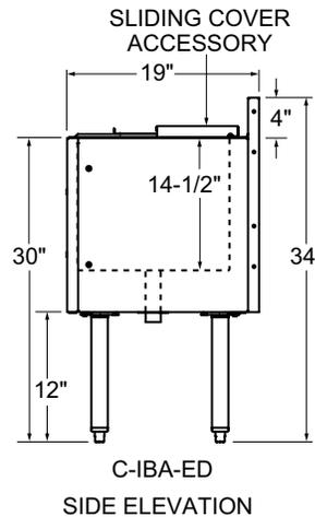
NOTE: Ice bins intended to store potable ice must be ordered with an ice bin cover to maintain the sanitation listing
