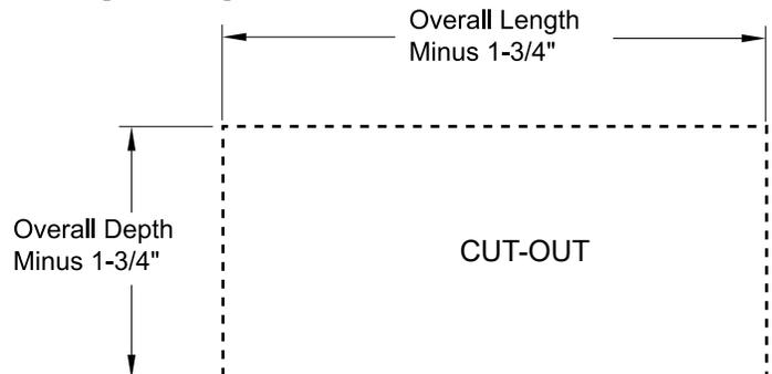
EXAMPLE: A DI-DP12X24 which measures 12" x 24" would require a cut-out size of 10-1/4" x 22-1/4"
